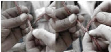
Put the other rope end through the loop and check the rope tension.
