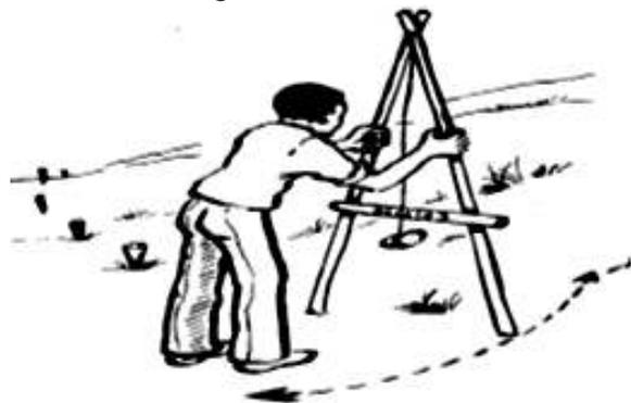
**Figure 2.9: Marking grade lines with an A-frame**
