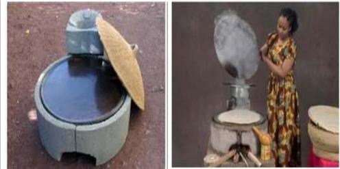
**Tikikil Stove:** a portable HH cook stove made of galvanized sheet metal with a ceramic liner. It saves up to 50% of fuel compared to the three-stone open fire; its heat efficiency is around 28%.
