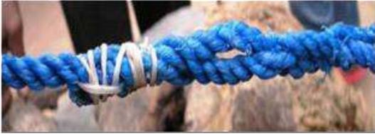
If nylon rope is used instead of PP, it is recommended to seam the end of the loop to avoid disconnection of the loop (nylon tends to slip)
