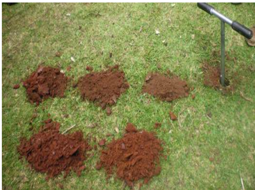
Figure 4-1: Auger-hole samples with arranged based on soil depth & other observed characters
