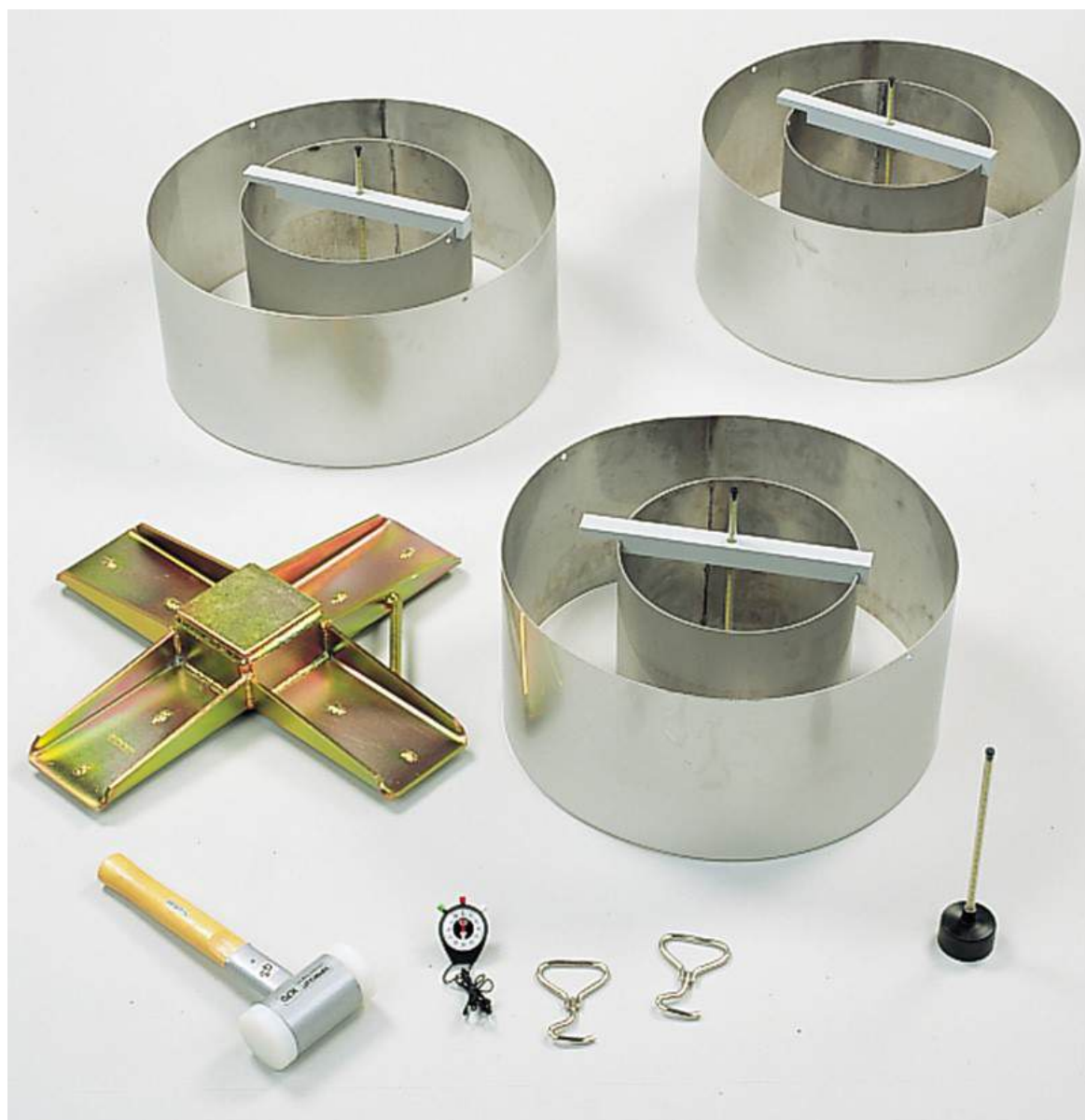
Figure 4-6: Double Ring Infiltrometer with Accessories
